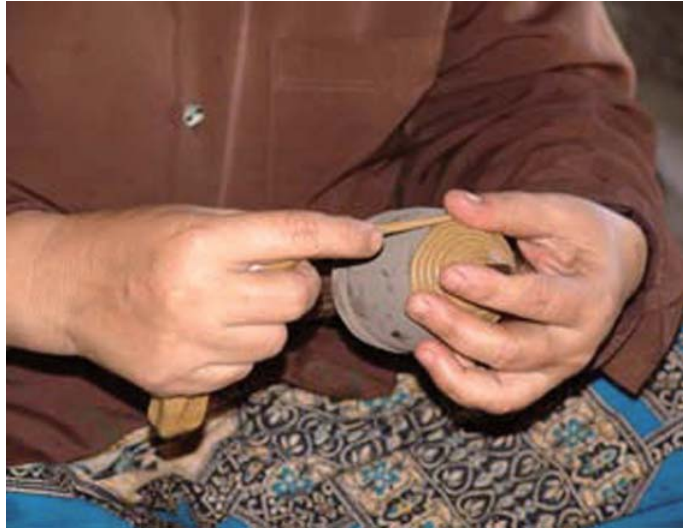
Clay model coated with molten wax
