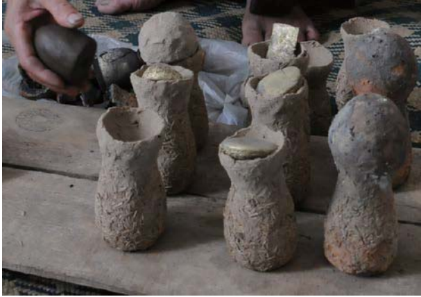
Molten brass alloy poured in the hollow ceramic shell mould and left to dry
